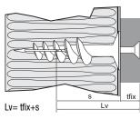
$\label{eq:s} \begin{array}{ll} s & = \mbox{ minimum insertion depth of screw in plug} \\ tfix & = \mbox{ fixing thickness} \end{array}$
